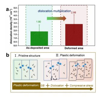
**Fig. 4 a** Statistical results of dislocation density before and after deformation in TiMoN coating. **b** Schematic illustration of deformation mechanisms of hard-yet-tough TiMoN system
