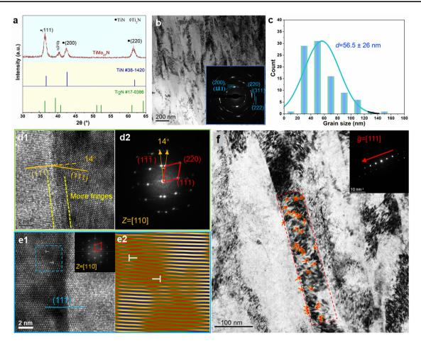
**Fig. 1** a XRD pattern of the as-deposited TiMo<sub>27</sub>N coatings; **b** BF TEM morphology of TiMo<sub>27</sub>N coating; **c** grain size distribution; **d** evidence of LAGB by atomic HRTEM image and SAED patterns; **e1** rotation GB with in-plane coherent GB but out-of-plane misorientation; **e2** corresponding IFFT; **f** identifying multiple nanoscale dislocation conserved by high-energy deposition through two-beam BF imaging under g = [111]
