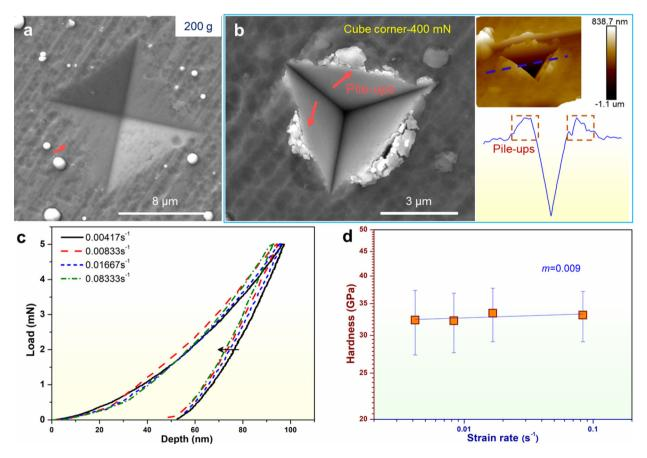
**Fig. 2** a Vickers print under 200 g showing a nearly crack-free except for a narrow and small one pointed by red arrow. b Morphology of cube corner under 400 mN. Surface and line scan clearly show pile up at the edges. c Representative load–depth curves of TiMoN coatings taken from load control mode. The arrow indicates the rising strain rate. d log–log plotting of hardness as a function of strain rate. The slope represents strain rate sensitivity, *m*
