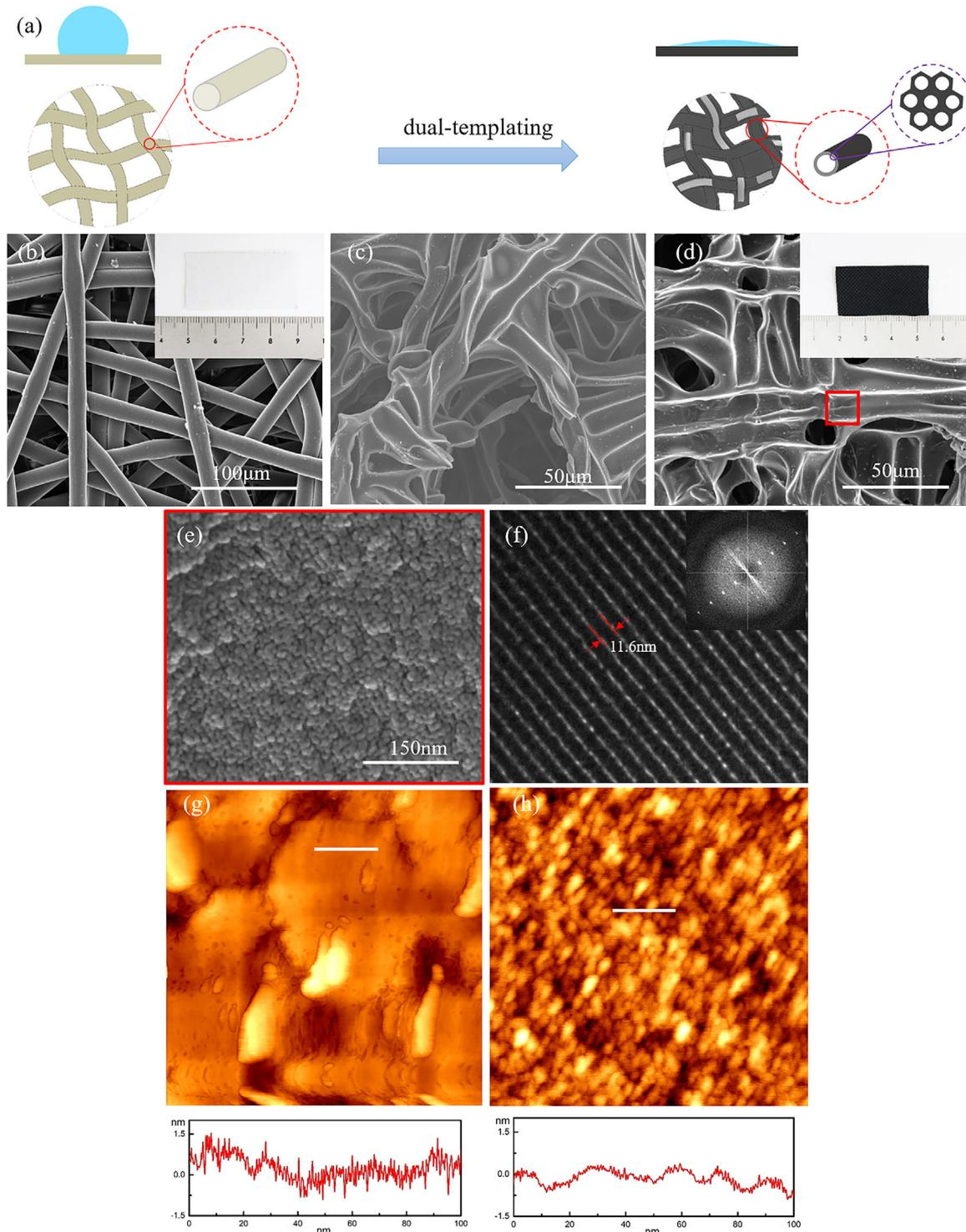
**Figure 1.** a) Scheme for comparison in structure between pristine PET and HC-PET fabrics; SEM images of b) pristine PET, c) C-PET sheet and d) HC-PET; e) locally magnified HC-PET fiber over a large domain; f) TEM and the corresponding fast Fourier transform (FFT) image; AFM profiles of g) C-PET, and h) HC-PET.
