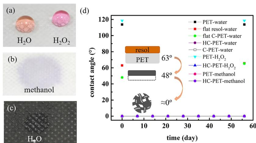
**Figure 3.** a) Water and  $H_2O_2$  liquid drops and b) methanol on the pristine PET; c) spread water drop on HC-PET; d) the CAs of different liquids on various samples in ambient condition.
