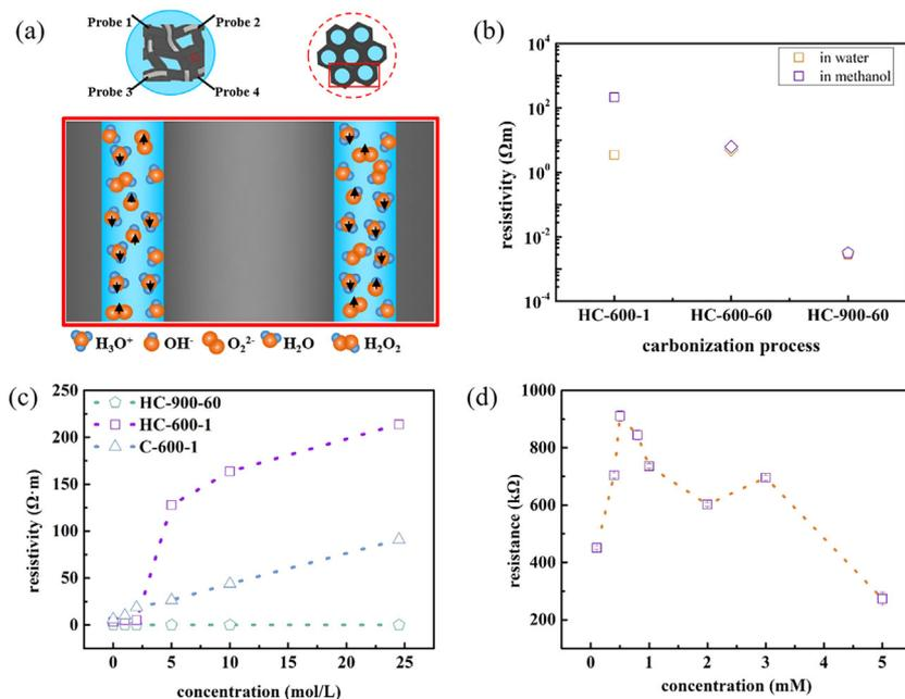
**Figure 5.** a) The scheme for liquid concentration detection; b) HC-PET sheets produced from different carbonization processes for water or methanol; c) resistivity changes of different porous materials in methanol solutions with different concentration; d) resistivity changes of HC-600-1 in  $H_2O_2$  solutions with different concentration.
