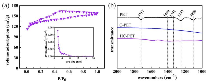
**Figure 2.** a)  $N_2$  adsorption–desorption isotherms of the HC-PET sheet; b) FT-IR data of PET, C-PET, and HC-PET fabrics.
